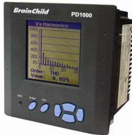
PD1000 power transducer is designed for continuous monitoring of 3 phase system. All essential power parameters including current, voltage, power, active and reactive energy are integrated in a single meter. Its bi-directional energy measurement and harmonic analysis function makes PD1000 suitable for modern industrial power management. The built-in Ethernet and rich communication abilities enable PD1000 to be easily connected with most modern third-party SCADA systems.
